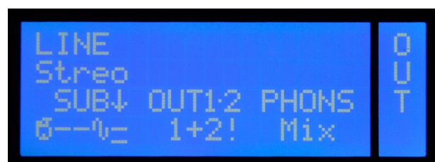
Busses 1 and 2 are assigned to OUT1 & 2
